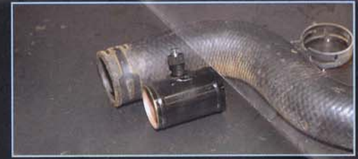
▲ Redarc sensor in our own pipe insert.
