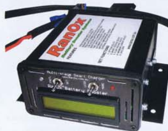
Clockwise from top: The Redarc 12 volt DC-DC alternator charger charges at up to 20 amps; external views of the RanOx DC-DC multi-stage battery booster; Redarc's BMS1215 fitted for testing and appraisal in the author's Nissan 4.2 litre TD Patrol.
