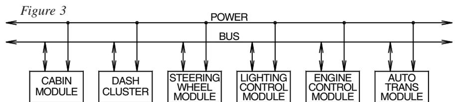
performing self-diagnostics, and transmitting their operating conditions around the Bus for all to know. Imagine now you want to add say a reverse sensor. No problems, just connect it to the data bus, define what messages this new module needs to receive and transmit and it is done!
