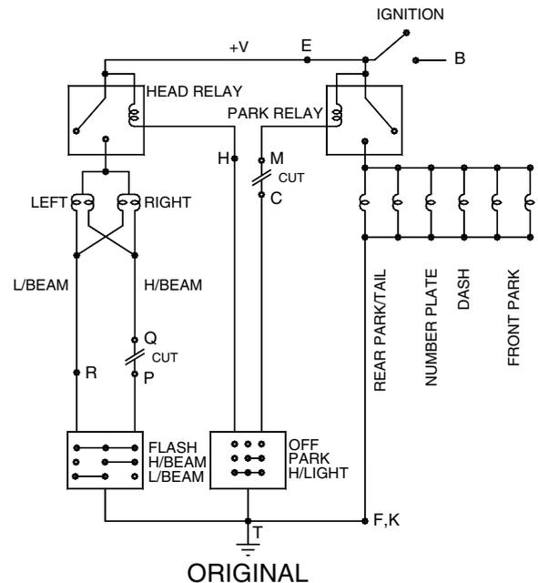
2. The rear tail light circuit can be isolated from the whole park light circuit. This can generally be done by simply cutting into the tail feed to the rear of the vehicle.
