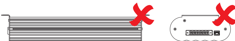
Figure 2.2.1.3 - Do NOT mount the unit upside down
