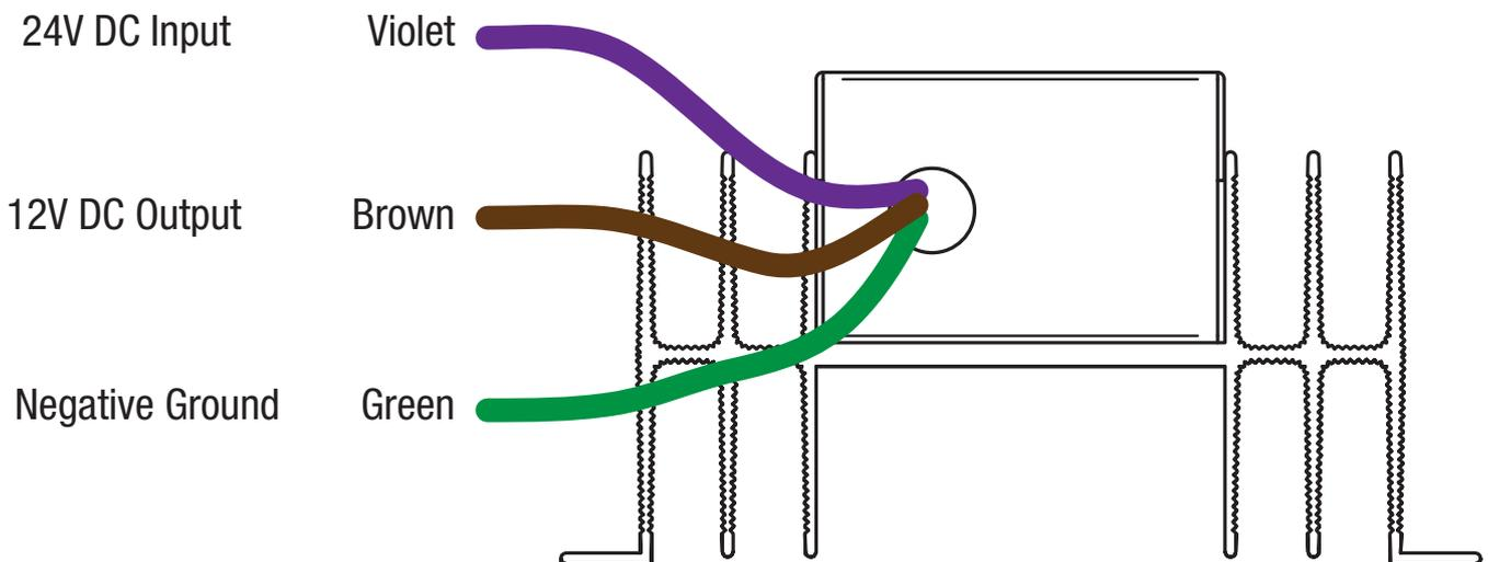
The GREEN WIRE must be connected first on installation and removed last when disconnecting. Failure to do so could void warranty.
